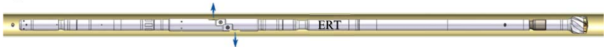
Figure 5b – The first ball is dropped and seated in the perforator to redirect flow out of the perforator
