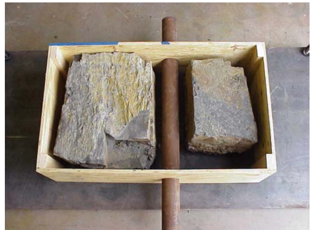
Figure 3 – Casing and Shale Samples within test assembly
