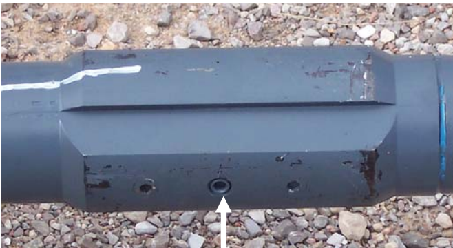
Figure 6 – Perforator dressed with two 0.125inch Orifices
