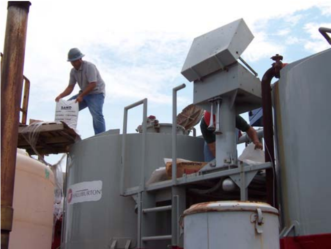
Figure 5 – Batch mixer used for sand slurry mixture
