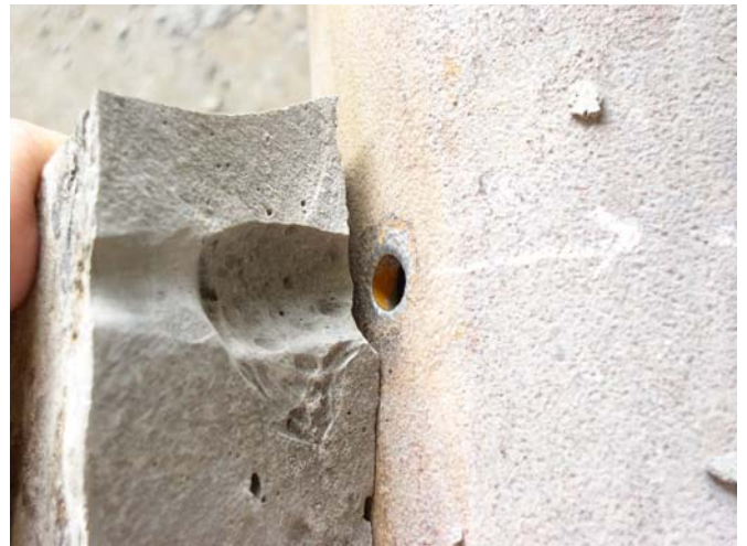
Figure 9 – Tear Drop Pattern of Erosion Effects
